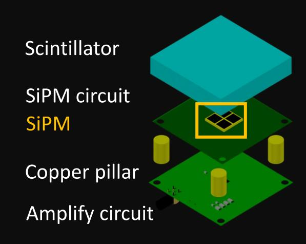
Our detector is made of a scintillator, a SiPM circuit, and an amplify circuit[2]. When charged particles hit the scintillator, it would emit photons and be caught by the SiPM, a light sensitive device, transforming the light signal into the electric signal. Since the original signal is in nano-second scale, a circuit of amplification and delay is necessary. For the sake of better expression, we name the detector, AW(阿瑋).
