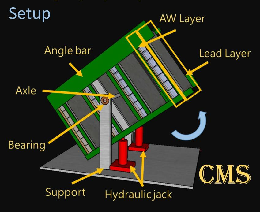
According to the signal on each layer, we can reconstruct the direction of the particle.
