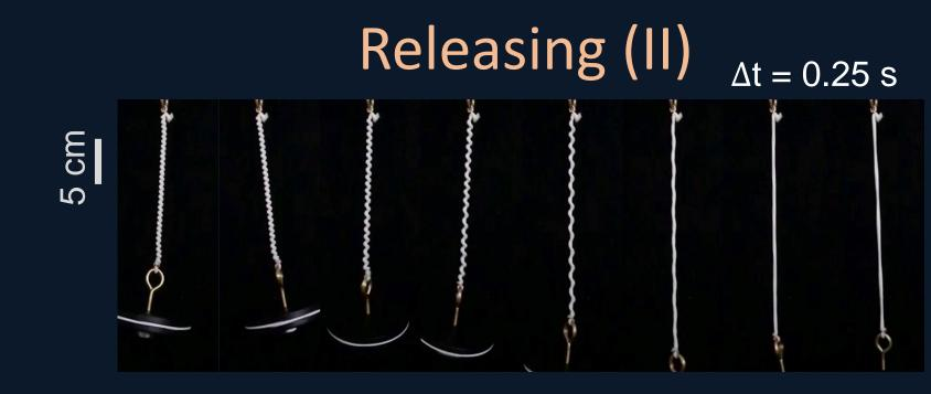
After the whole filament becomes solenoid, it starts to unwind solenoid evenly because the filament tends to be straight.
