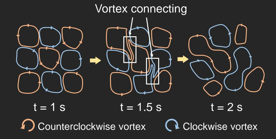
Vortices with same rotational direction merge together because the velocities between vortices are canceled out.
