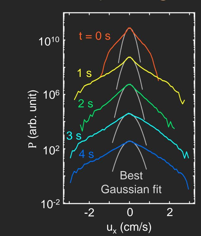
The non-Gaussian tails are formed of as time increases the increased velocity. However, histogram becomes narrow at t = 2 s which is caused by the vortices merging.
