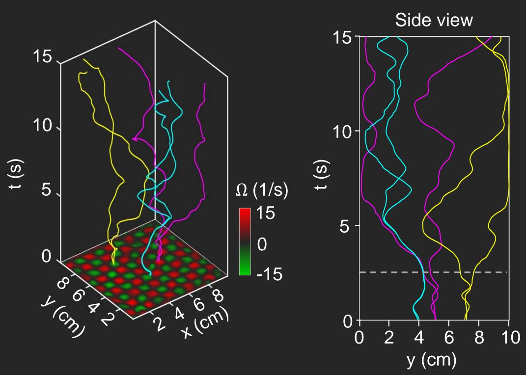
The particles are trapped in the same vortex at the single-scale state. When the system becomes turbulence, the particles will travel to different vortices. Gray dashed lines indicates the transition time to the turbulent state.
