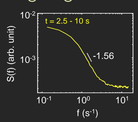
Lagrangian velocity spectra of particle trajectories follow power-law decay, which represent turbulent like particle motion.
