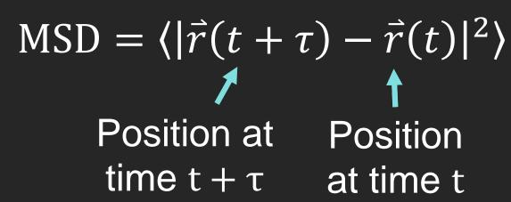
MSD slope > 1 meaning that particles tend to maintain moving direction. MSD slope < 1 indicating that particles are trapped.
