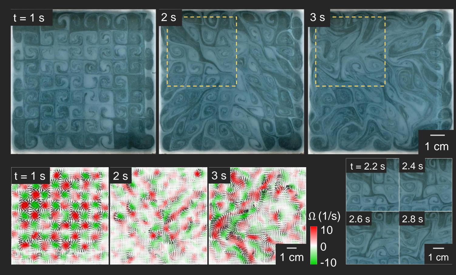
The system is turned on at t = 0 s. At t = 1 s, the system forms square lattice, in which the velocity and vorticity of vortices are similar. At t = 2 s, the vortices start to merge with decreased velocity and vorticity, which is the transition process between single-scale and turbulent states. At t = 3 s, the multiscale vortices are generated.
