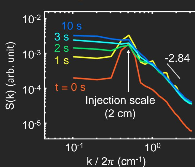
At t = 0 s, the spatial spectrum shows the peak at 2 cm, indicating the injection scale of the system. With increasing time, the spectra transit to power-law decay. It means the vortices are generated over a wide range of scales in the turbulent state.
